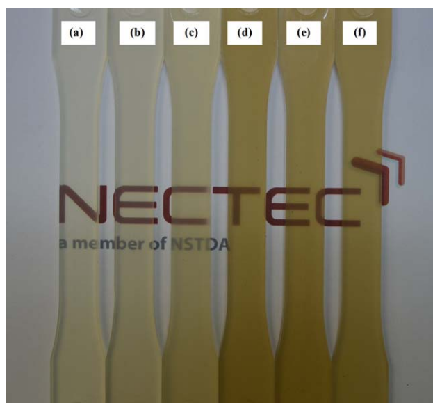
Figure 7. Tensile test specimen of (a) PLA, (b) PLA/EPO, (c) PLA/EPO/0.2 wt % GP, (d) PLA/EPO/0.4 wt % GP, (e) PLA/EPO/0.6 wt % GP, and (f) PLA/EPO/0.8 wt % GP. [Color figure can be viewed in the online issue, which is available at wileyonlinelibrary.com .]
